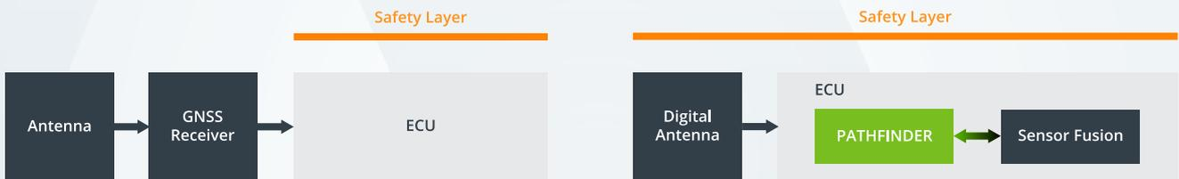
**Traditional Setup.** A dedicated hardware GNSS receiver plus antenna results in a complex system architecture. An integrated supervision of the receiver performance is not possible.
